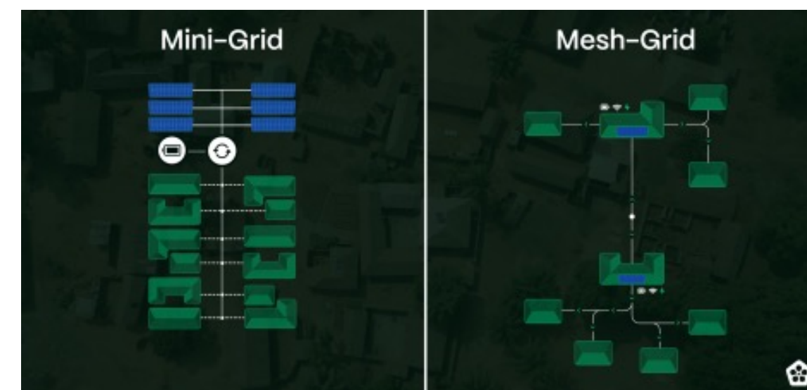
Figure 1. Visual of PV, inverter and battery-system locations in a mini-grid (left) versus mesh-grid system configuration. Graphic provided by Okra Solar.
